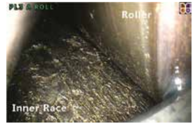
Figure 5: Romax Inspection Showing Failed Main Bearing
