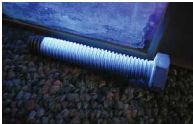
Images 3 and 4: A bolt coated with the Illumi-Layer™ CEN coating containing light-emitting particles and photographed under normal light (left) and ultraviolet light (right) to illuminate for authentication and indication
