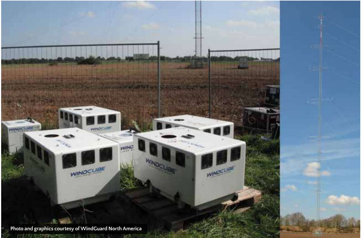
Figure 1: Calibration test field of Deutsche WindGuard. Left: Enclosure with tested LiDARs in front and the base of the 135 m high reference met mast in the back. Right: Wide shot of the reference mast from a view angle opposite of the one on the left.
